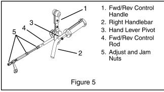
Connect the Fwd/Rev and Hi-Lo gear control rods to the tractor and their respective handles using bushings, 1/4-20 x 1.5 bolts, .281 x .625 x .065 x flat washers and 1/4-20 locknuts. See the gear shift control and direction control. (Figure 1) and (Figure 5) Adjust per Owner/Operator Manual.
